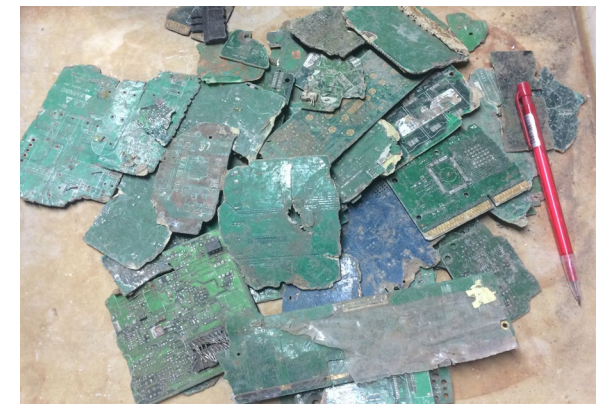
Typical post-shredder PCBs
